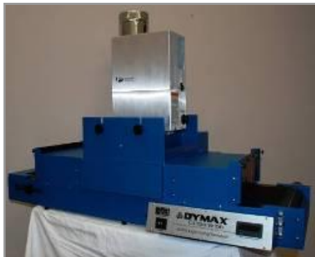
Figure 5. Conveyor with Lamp(s) Installed
