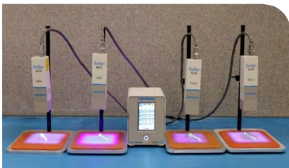
Figure 2. BlueWave® MX-250 System with 4-Channel Controller
