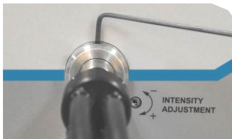
Figure 7. Gently Tighten Setscrew on Lightguide Mount with Hex Wrench
