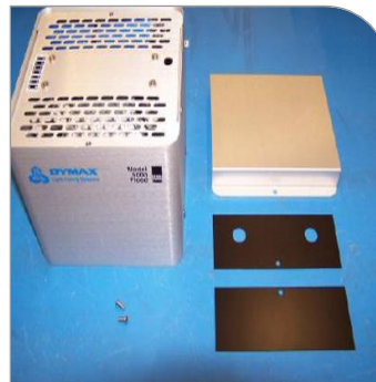
Figure 1. 5000-EC with Cover Removed & Temperature Control Kit
