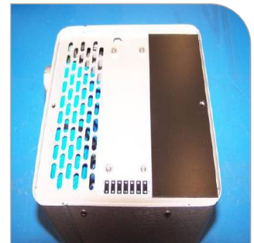
Figure 2. One Temperature Control Plate Installed
