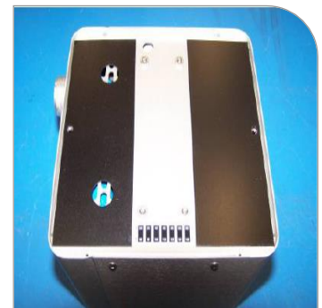
Figure 4. Two Temperature Control Plates Installed
