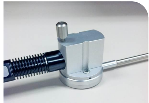
Figure 17. Insert LED Head into Optical Adapter
