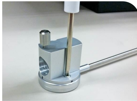
Figure 16. Attach Optic Adapter to Detector
