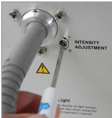
**Figure 8. Intensity Adjustment with Knob**
