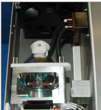
**Figure 21. Lift Bulb Mounting Bracket**
