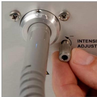
**Figure 9. Intensity Adjustment (Interior View)**
