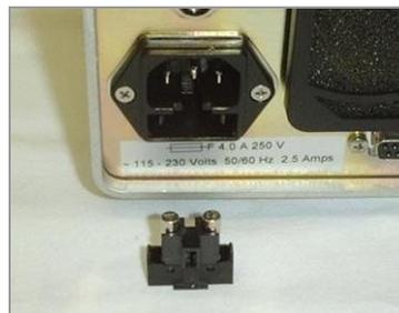
**Figure 19. Fuses Removed from Holder**
