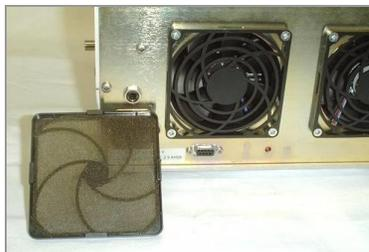
Figure 16. Cooling Fan Cover and Filter
