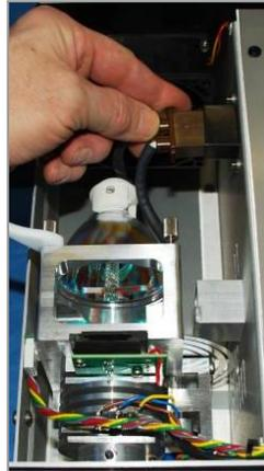
**Figure 26. Tighten Mounting Bracket Thumbscrews**
