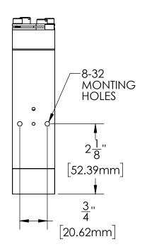
T15859 = 1/4" NPT W/ VITON SEALS T15853 = 1/4" NPT W/ TEFLON SEALS T15855 = 1/4-28 W/ TEFLON SEALS
