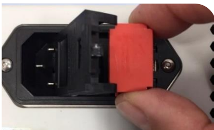
Figure 43. Remove Fuse Holder
