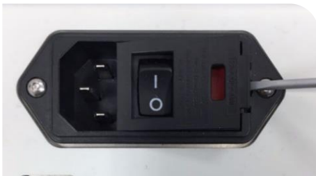
Figure 41. Open Fuse Cover
