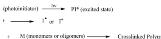
Figure 1. Polymerization Steps in Light Curing
