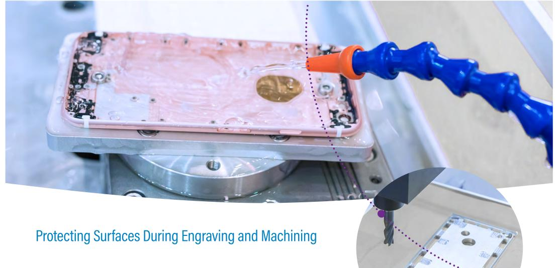
One of the strengths of light-curable maskants is their durability. Cured maskants are resilient enough that they can be machined through, without the remaining mask lifting and compromising protection. They can also withstand various water-soluble and oil-based coolants used in machining. This creates clean, crisp edges and can be beneficial when engraving logos, safety warning, or other items on parts or when machining out areas for buttons, speaker areas, and other jacks.
